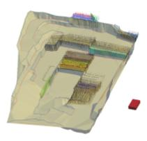
Thus all the elements are available to establish a safe fire plan, guaranteeing optimum mass distribution, while respecting the environment by limiting the vibrations. A hole-by-hole loading plan for quality mining can be obtained in this way. All shooting plans are incorporated into a global topographic model for continuous tracking of the mining activity.
