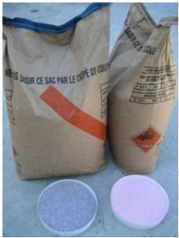
**The NITRO D8** is a standard ANFO. Safe yet powerful, it is used in quarries and civil engineering projects, in combination with traditional cartridge explosives. NITRAL is an aluminium-doped nitrate. This strong addition of energy makes it particularly effective for hard rock blasting and for good blast shearing design.
